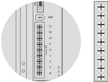
Pic 4.3 Main Circuit Terminal
