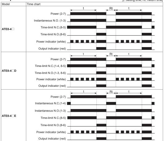
When time-limit of ATE8-4□, ATE8-4□E is set to 0, time-limit contact operates within 30ms right after instantaneous contact operation.
