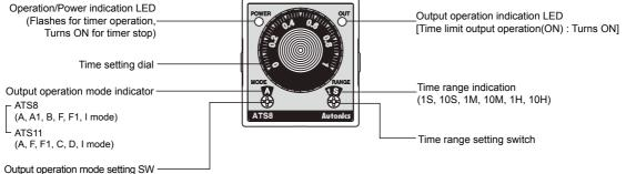
XTurn the time range setting switch and the output operation mode setting switche to clockwise(CW) direction.
