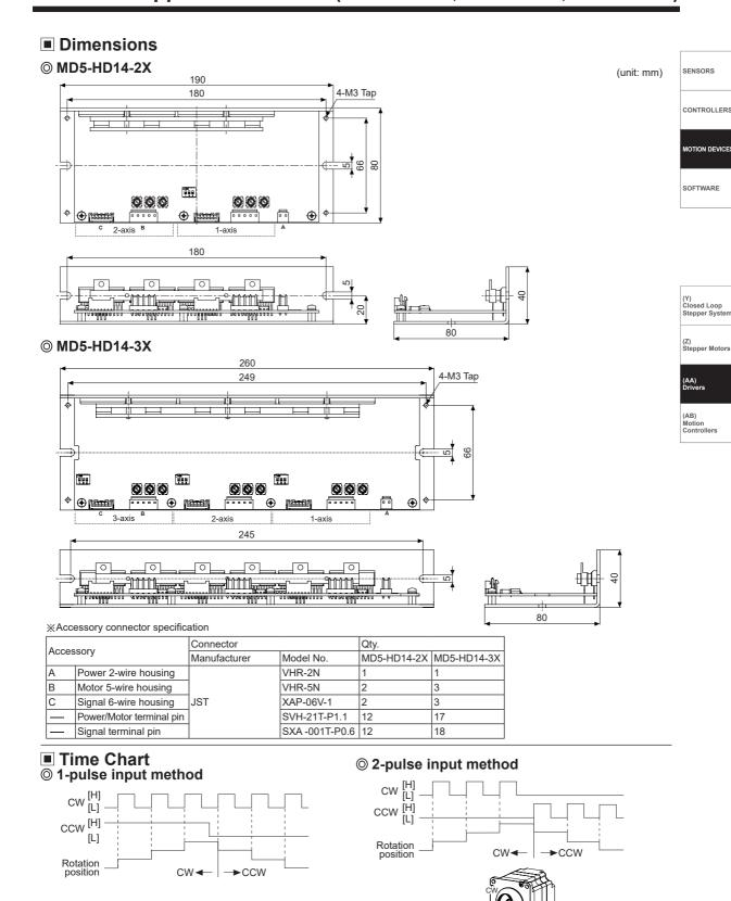
XDo not input CW, CCW signals at the same time in 2-pulse input method.
