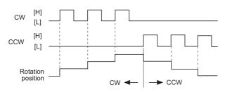
\*\*Do not input CW, CCW signals at the same time in 2-pulse input method.
