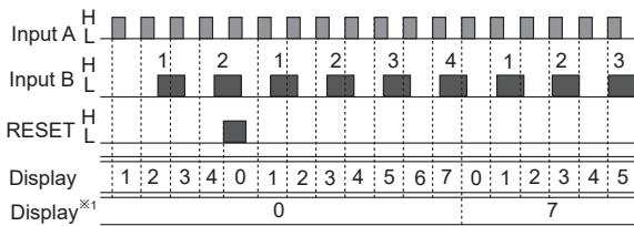
$\times$ 1: When the display cycle [ $d1\ 5PL$ ] setting is OFF, it will maintain the quantity of input A until the value of input B reaches the setting value B[ $\square\ U.n.b$ ].
