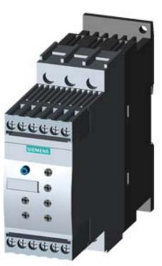
SIRIUS soft starter S0 32 A, 15 kW/400 V, 40 °C 200-480 V AC, 110-230 V AC/DC Screw terminals
