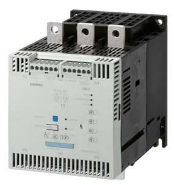
SIRIUS soft starter S12 432 A, 250 kW/400 V, 40 °C 200-460 V AC, 230 V AC Screw terminals !!! Phased-out product !!! Successor is SIRIUS 3RW5, Preferred successor type is >>3RW5076-6AB14<<
