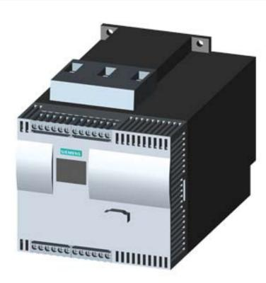
SIRIUS soft starter Values at 400 V, 40 °C standard: 93 A, 45 kW Inside-delta: 161 A, 90 kW 200-460 V AC, 230 V AC Screw terminals !!! Phased-out product !!! Successor is SIRIUS 3RW5, Preferred successor type is >>3RW5527-1HA14<<
