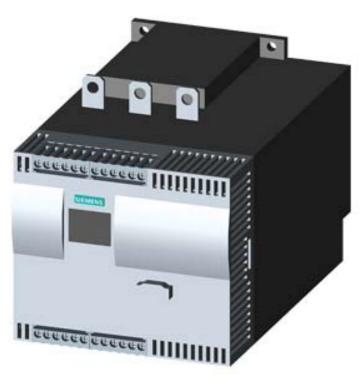
SIRIUS soft starter Values at 400 V, 40 °C standard: 134 A, 75 kW Inside-delta: 232 A, 132 kW 200-460 V AC, 230 V AC Screw terminals !!! Phased-out product !!! Successor is SIRIUS 3RW5, Preferred successor type is >>3RW5535-6HA14<<
