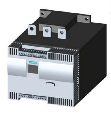
SIRIUS soft starter Values at 400 V, 40 °C standard: 356 A, 200 kW Inside-delta: 617 A, 355 kW 200-460 V AC, 230 V AC Screw terminals !!! Phased-out product !!! Successor is SIRIUS 3RW5, Preferred successor type is >>3RW5546-6HA14<<
