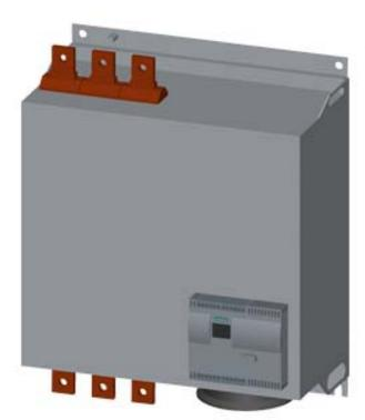
SIRIUS soft starter Values at 400 V, 40 °C standard: 551 A, 315 kW Inside-delta: 954 A, 560 kW 200-460 V AC, 230 V AC Screw terminals !!! Phased-out product !!! Successor is SIRIUS 3RW5, Preferred successor type is >>3RW5548-6HA14<<
